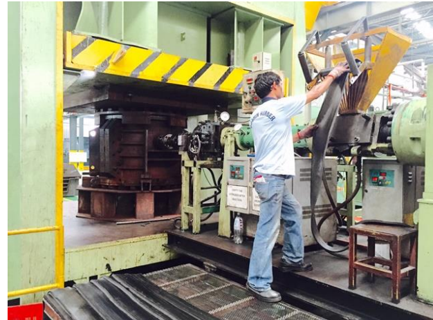
INJECTION TO FENDER AT 1500KG/HR
