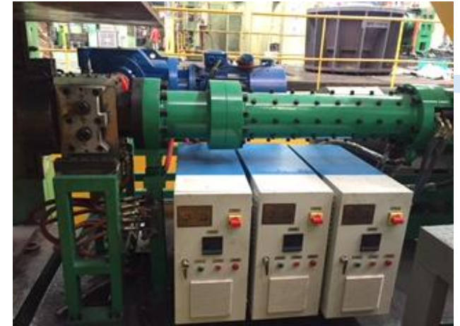
3 UNITS GEAR PUMP EXTRUDER 1500KG/HR
