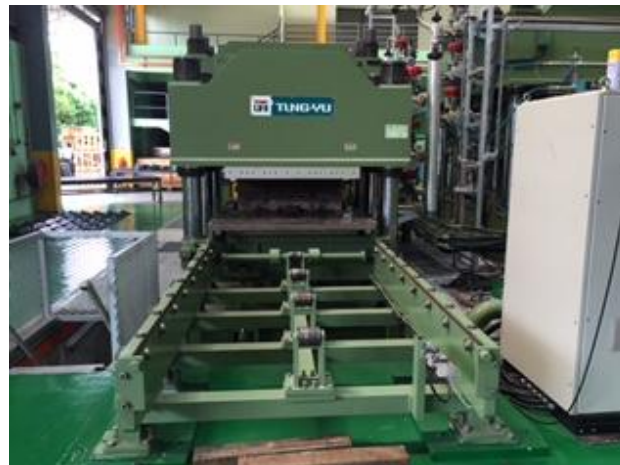
1200 TONS COMPRESSION PRESS 1.2M X 2.2M
