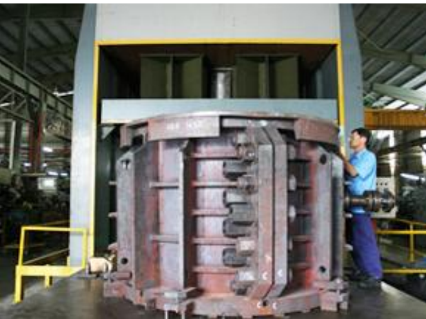
2000 TONS CLAMPING MACHINE 3.5M X 3.5M X 3.0M DAYLIGHT
