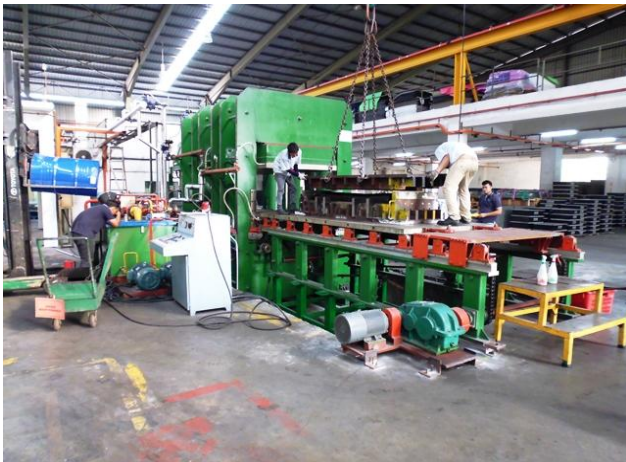
2000 TONS COMPRESSION MACHINE 1.5M X 3.5M
