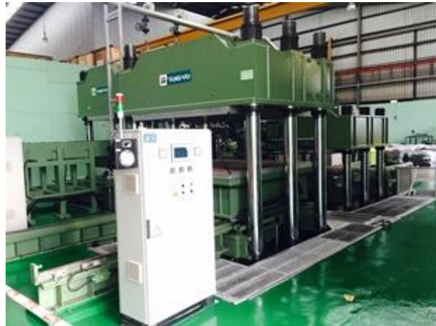
2000 TONS COMPRESSION MACHINE 2.2M X 2.2M
