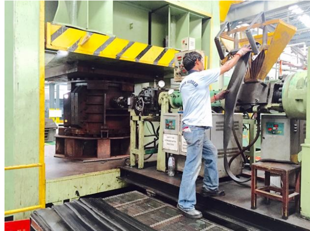
INJECTION TO FENDER AT 1500KG/HR
