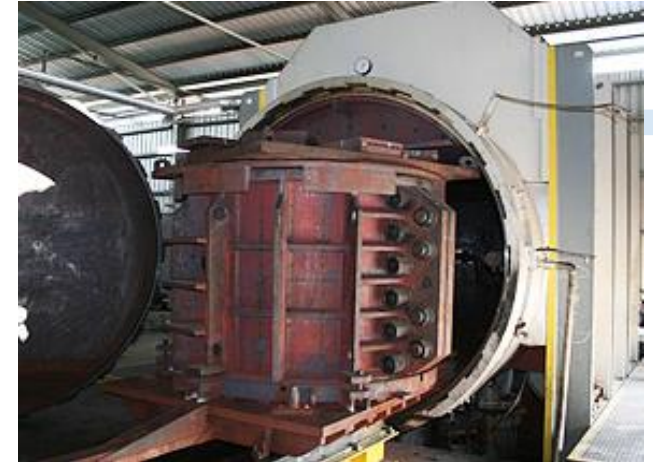
1800 TONS HYDRAULIC BUILT INTO AUTOLAVE FOR CURING
