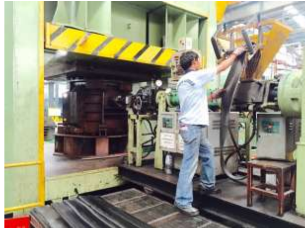
INJECTION TO FENDER AT 1500KG/HR
