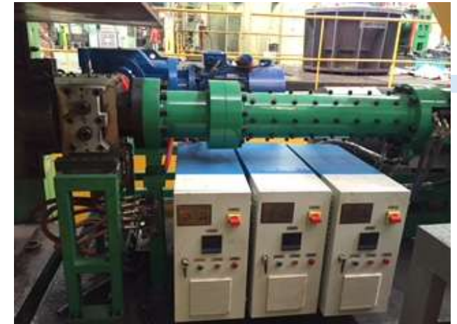
3 UNITS GEAR PUMP EXTRUDER 1500KG/HR
