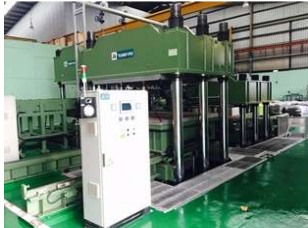
2000 TONS COMPRESSION MACHINE 2.2M X 2.2M
