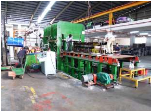
2000 TONS COMPRESSION MACHINE 1.5M X 3.5M
