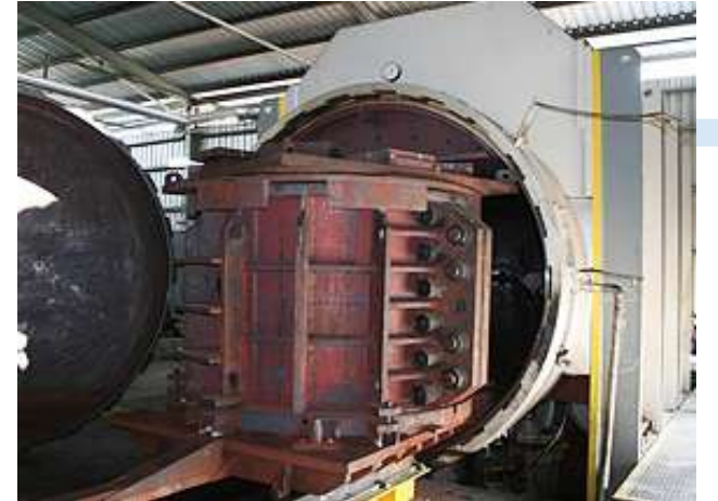
1800 TONS HYDRAULIC BUILT INTO AUTOCLAVE FOR CURING
