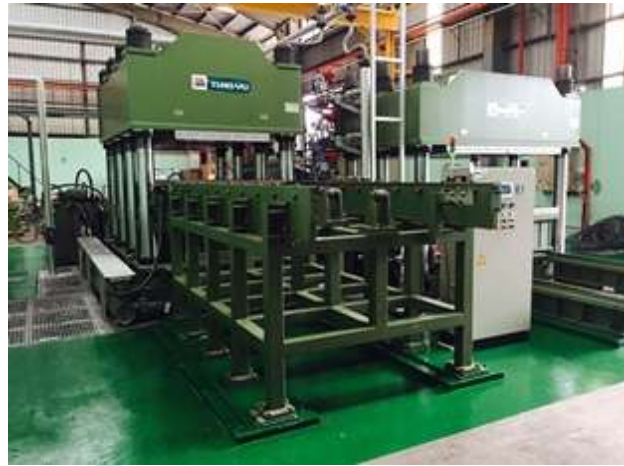
2000 TONS COMPRESSION MACHINE 1.2M X 3.2M
