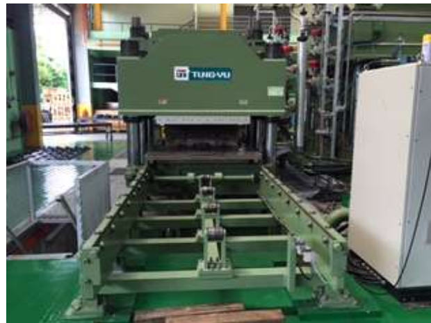
1200 TONS COMPRESSION PRESS 1.2M X 2.2M
