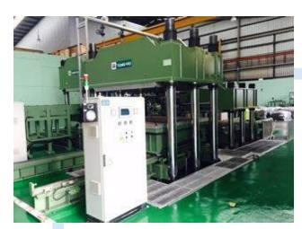
2000 TONS COMPRESSION MACHINE 2.2M X 2.2M
