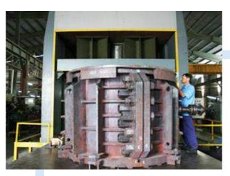
2000 TONS CLAMPING MACHINE 3.5M X 3.5M X 3.0M DAYLIGHT
