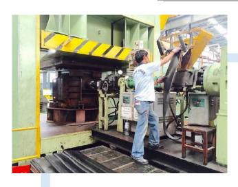
INJECTION TO FENDER AT 1500KG/HR
