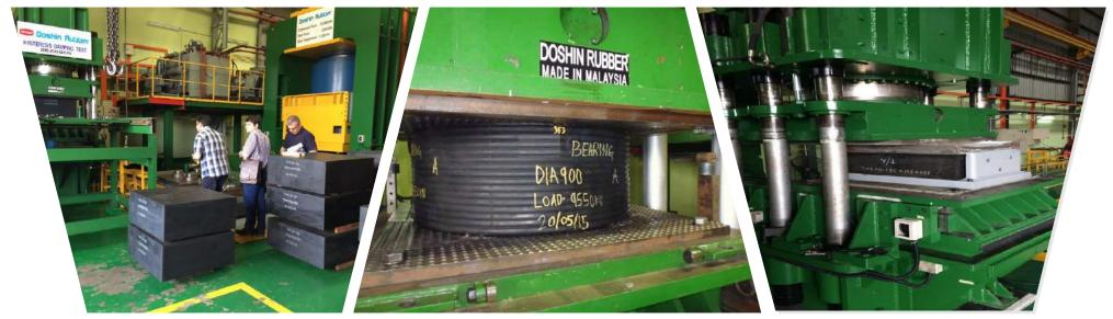
HYSTRESIS DAMPING TESTING FOR STRUCTURAL BEARINGS AND SEISMIC ISOLATORS
