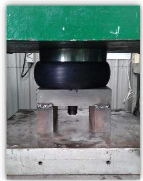
Vertical Load: 1,000KN Shear Load: 100KN
