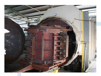
1800 TONS HYDRAULIC BUILT INTO AUTOLAVE FOR CURING
