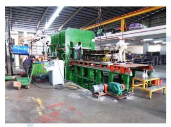
2000 TONS COMPRESSION MACHINE 1.5M X 3.5M
