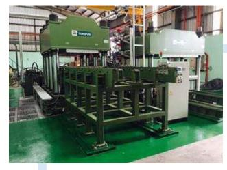
2000 TONS COMPRESSION MACHINE 1.2M X 3.2M
