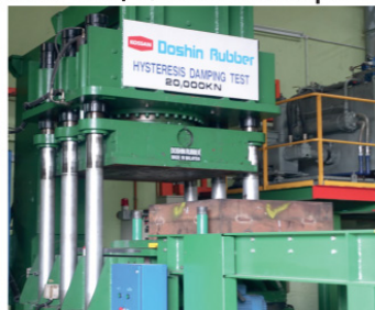
➤ Compressive load test (20.000 kN, shear force 2000 kN)
