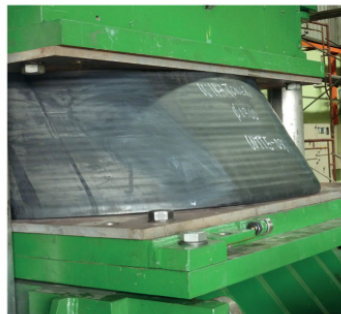
➤ Test rig for isolators testing (50000 kN compressive load, 5000 kN shear load, +/- 1000 mm displacement)
