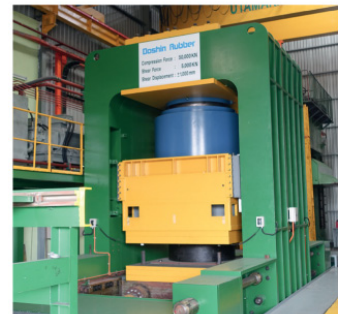
➤ Test rig for isolators testing (50000 kN compressive load, 5000 kN shear load, +/- 1000 mm displacement)
